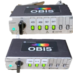
6 & 7 Laser Power Supply 2 Boxes
